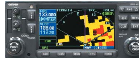
Garmin 400/500 Series units with main software version 5.10 or above, along with corresponding hardware upgrades, include Garmin TERRAIN as a standard feature.
